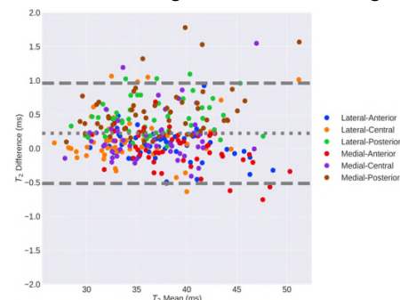
Figure 2: Bland-Altman analysis of T_2 estimates from deep-learning super-resolved scan shows minimal bias ( \sim 0.25 ms) and strong concordance to ground truth.
